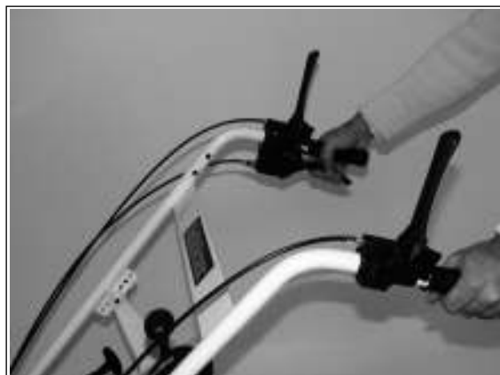
2) The machine will drive backwards for as long as you hold the switch lever down.
