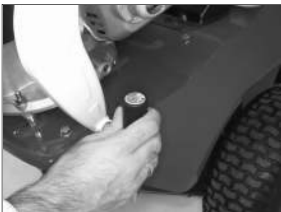
3) Gear selection lever to front: 3rd gear = fast
