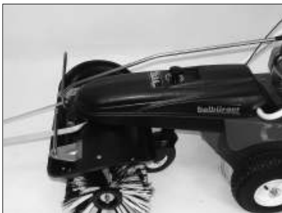
1) Position of lashing strap at front.
