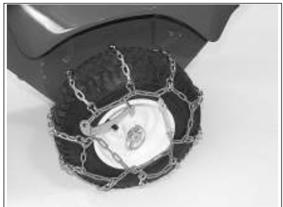
4) Push the wheel with fitted snow chain over the axle and then secure with the cotter pin. Fit the second snow chain in the same way.
