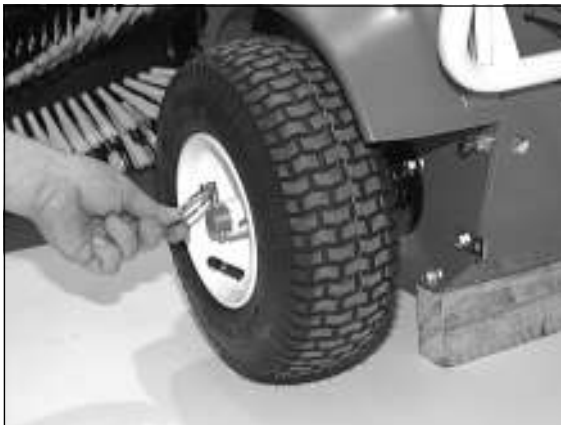
1) First raise the machine on wooden blocks and then remove the wheel.
