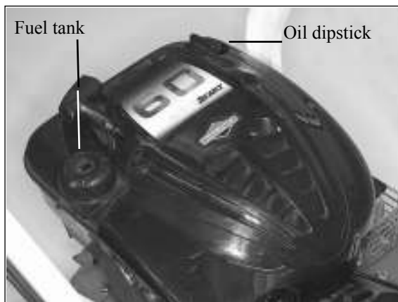
1) Fuel and oil tanks on B&S motor
