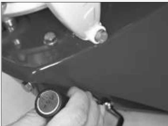
1) Gear selection lever back: 1st gear = slow
