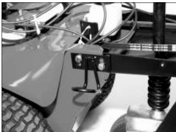
4) Properly installed towing eye. On the opposite side, proceed as follows.
