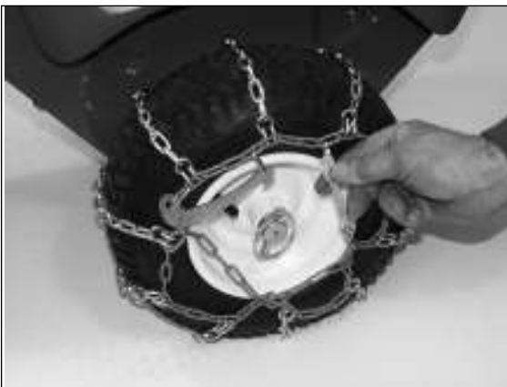
3) The chain put around the wheel and tighten the clamp across the wheel and hook.
