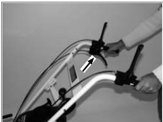
1) The bottom switch lever on the right-hand end of the handlebar selects reverse gear.
