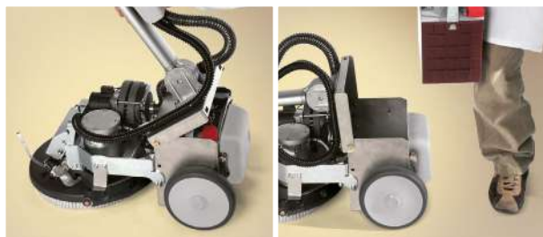
Vispa 35 B - Bs The battery compartment is easily accessible for quick battery replacement
